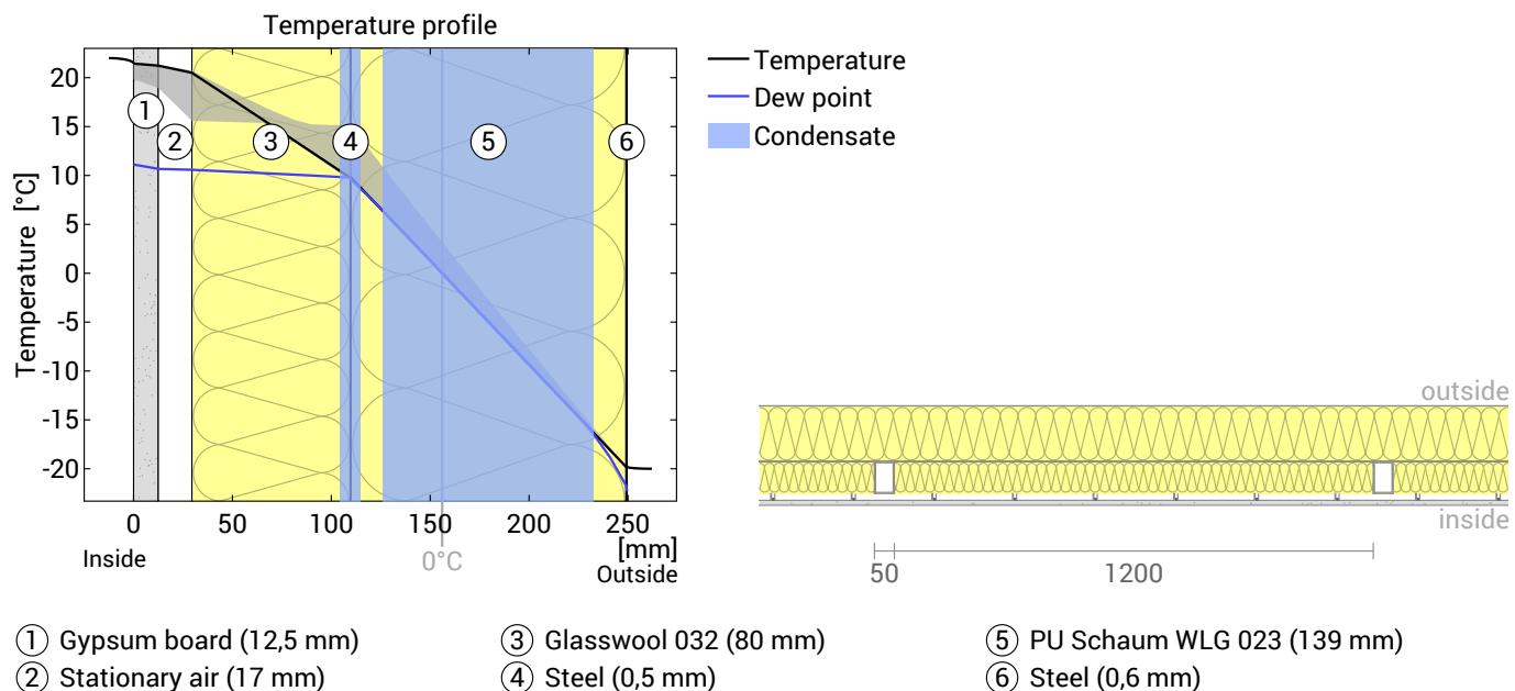
**Left:** Temperature and dew-point temperature at the place marked in the right figure. The dew-point indicates the temperature, at which water vapour condenses. As long as the temperature of the component is everywhere above the dew point, no condensation occurs. If the curves have contact, condensation occurs at the corresponding position.
