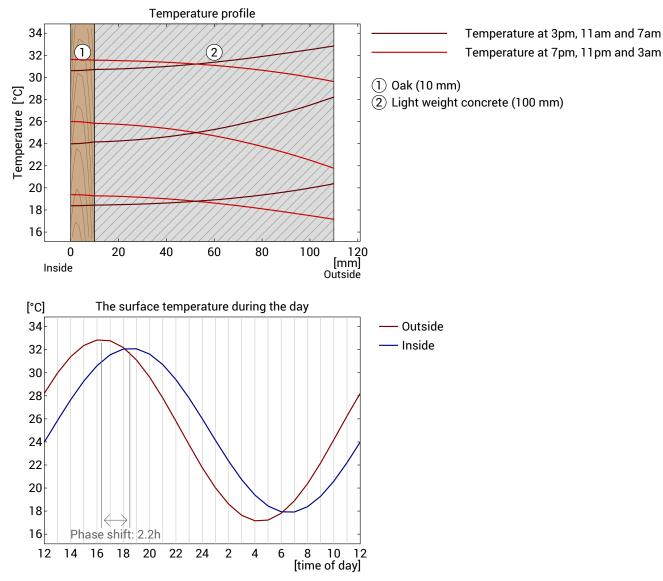
**Top:**Temperature profile within the component at different times. From top to bottom, brown lines: at 3 pm, 11 am and 7 am and red lines at 7 pm, 11 pm and 3 am.
