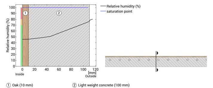
Notes: Calculation using the Ubakus 2D-FE method. Convection and the capillarity of the building materials were not considered. The drying time may take longer under unfavorable conditions (shading, damp / cool summers) than calculated here.
